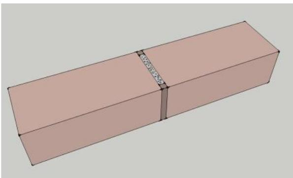
**Figure 13: External movement joint with compressible filter**
