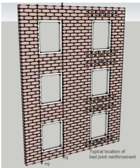
Areas of weakness also occur when the openings are wide in relation to their height or where large openings are positioned vertically above each other. In these instances vertical joints should be considered adjacent to the jambs or bed joint reinforcement introduced. See *Figure 10*.
